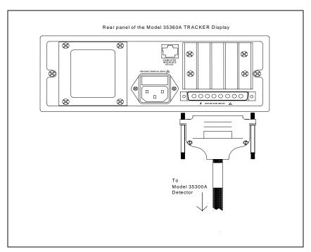
Figure 2-3. Connecting the Interface Cable to the Model 35300A Detector
